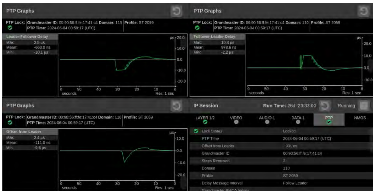
Figure 6. PRISM Offset from Leader PTP Graph for Test 6.
